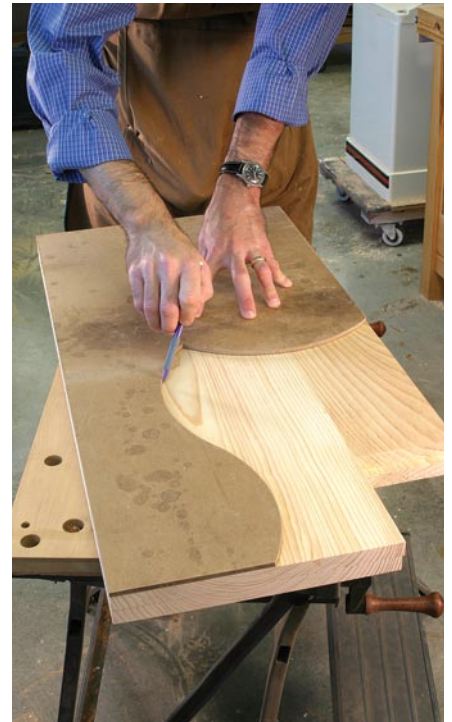
Watch those curves. A full-size template helps in many ways. It allows you to refine the design details, determine the finished sizes of key components and to lay out your cuts.
