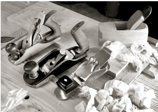
SMOOTHING PLANES ARE THE ELITE (and most demanding) planes in your shop. Shown is a Lie-Nielsen No. 4, a Veritas bevel-up smoother, a wooden-bodied Clark & Williams smoother, and my most guilty pleasure: a custom-made plane by Wayne Anderson (bottom right). Yes, it's a smoothing plane, too.
