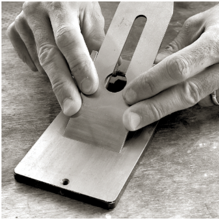
THERE ARE LOTS OF WAYS to get the proper camber on the iron for a jointer plane. Shown is the Odate crowning plate from Powell Manufacturing – essentially, it's a diamond sharpening stone that's concave in the middle.
