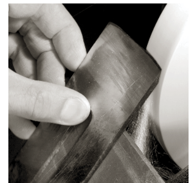
CAMBERING THE IRON on a fore plane is a task best handled on a bench grinder.
