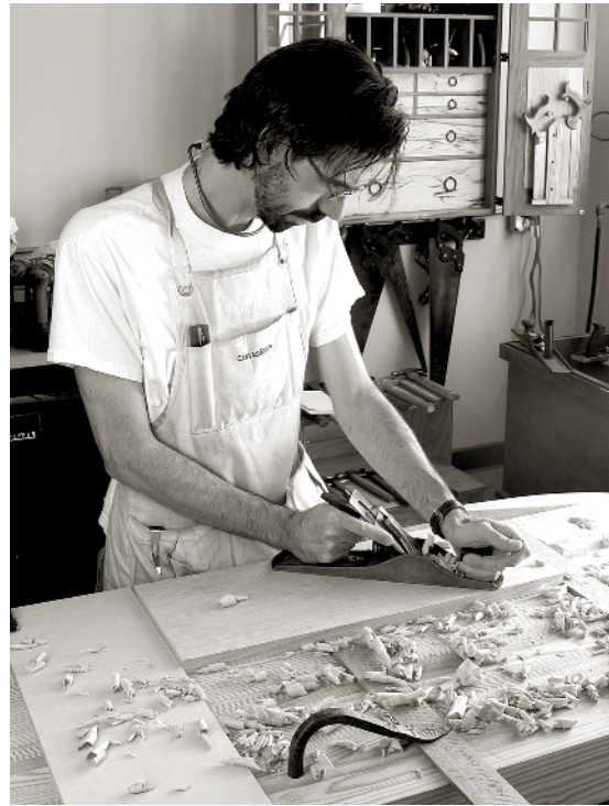
WORKING DIAGONALLY OR ACROSS THE work is the key to using the fore plane. The diagonal motion reduces tear-out and assists in truing the face.
