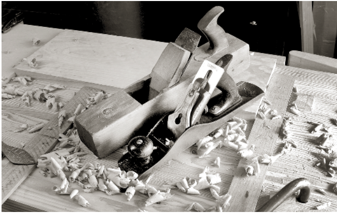
LIKE A POWERED PLANER, THE fore plane produces thick curls so it can rapidly reduce a board in thickness. Shown is my crusty-but-trusty Stanley No. 5 (some people call this a jack plane) and my sweet Scioto Works 16" wooden-stock fore plane.
