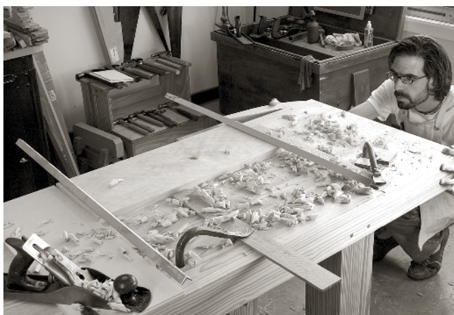
WINDING STICKS (I LIKE ALUMINUM angle) exaggerate any warp or high spots on the board's face. View the winding sticks so they are in line with one another.
