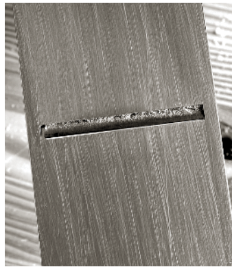
THE MOUTH OF THE JOINTER plane is a fine balance. You want it open enough to pass a fairly thick shaving, yet tight enough to limit tear-out as much as possible.
