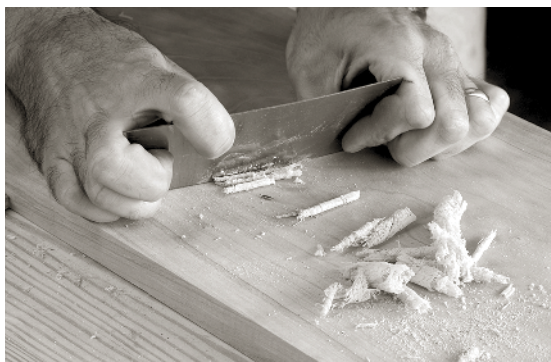
HAND SCRAPERS AND SANDING BLOCKS are an accepted and historically accurate way to prepare a piece of wood for finishing.
