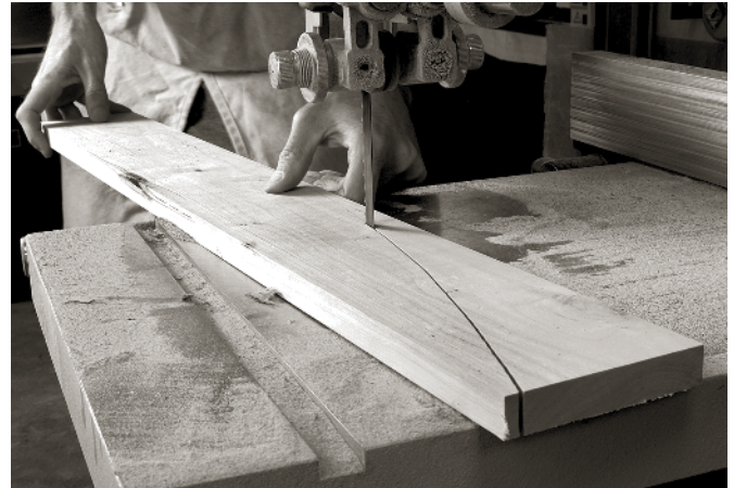
THE CONCEPT OF COARSE, MEDIUM and fine works with other operations as well. For cutting curves, think of your band saw as the coarse tool, your rasp as the medium tool and your spokeshave as the fine tool.
