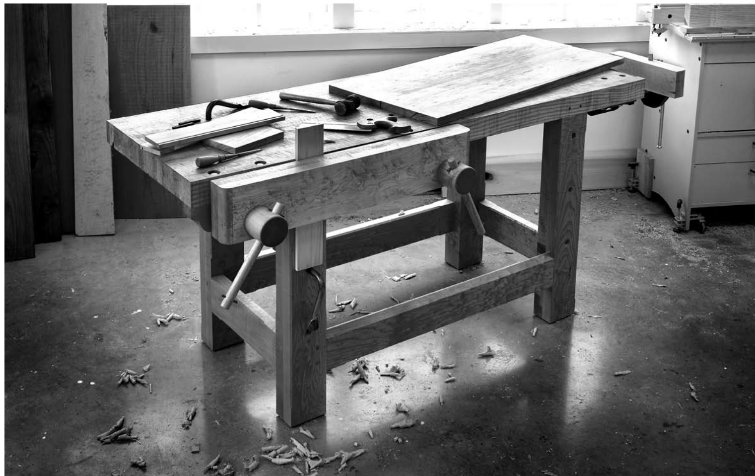
This 19th-century workbench can be built to be knocked down with bolts, or it can be built as a permanent addition to your shop, as shown here.
