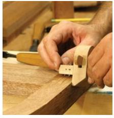
**Set, then reset.** I reset my marking gauge to mark out the mortise. Because the left and right legs differ slightly in thickness, this setting won't work on the opposite leg.
