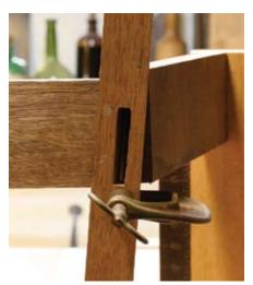
*In position.* I have the side seat rail positioned correctly. The exposed material to the right of the leg will get planed flush with the back leg later.
