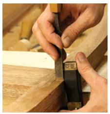
Chisels for marking. I flipped the leg over, and measured in from the bevel using the same chisel. I like using chisels as gauge blocks. In the 18th century, you'd be lucky to have a ruler with eighths marked on it. But even today, this helps eliminate measuring errors and when you can do it, you can mark and measure at the same time.
