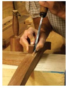
Jig - of sorts. I like to pare out the waste in my mortises. I squeezed my gauge block against the side of my mortise to help me maintain the correct angle. This is as close as I get to using jigs.
