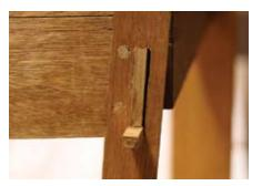
**Tough job.** This is the toughest joint in a chair full of tough joints. Something went terribly wrong marking out this tenon, but at least I got the rail positioned correctly! Turns out these tenons were typically wedged, but not with the massive <sup>1</sup>/<sub>4</sub>" block in this one. As bad as it looks now though, I'll bet it will look a lot better with a couple wedges and some leftover mahogany veneer from my standing desk. We may be surprised when it's done.
