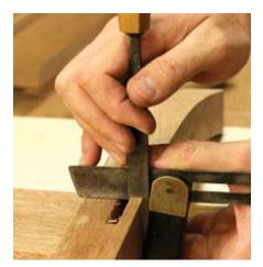
Just right. I placed my bevel gauge against the front face of the leg and measured over from the gauge to the mortise. This 1/2" chisel was just right.
