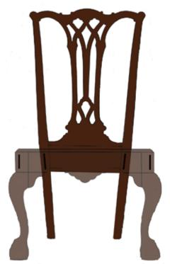
Simple structure. The basic structure of this sort of formal chair is simple enough. The seat frame is mortised and tenoned together. Knee blocks, glued in later, help visually blend the joint between the seat rails and the legs. They aren't structural. The picture above is missing glue blocks at the inside corners of the seat rails. I'll cover them in a future article.
