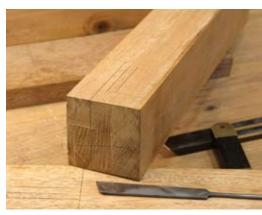
**Leg layout.** Mark the outer surfaces of the legs using the inner reference faces. The angle of the side seat rails must come from a full-sized drawing or existing chair.
