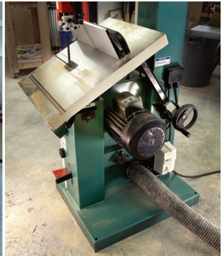
Two fine features. The table tilt mechanism is easy to adjust, and the foot-activated pedal is both a stop switch and blade brake.
