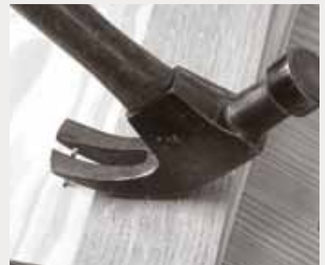
When using the claws of a hammer to extract a nail, always place a piece of scrap under the head to protect your work. Both hardwoods and softwoods can be damaged easily by the prying action of a claw hammer. And if you need more leverage, use a thicker scrap.
