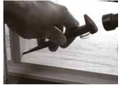
Toenailing allows you to nail joints from the inside of a project and to conceal the nail head in carcass construction.
