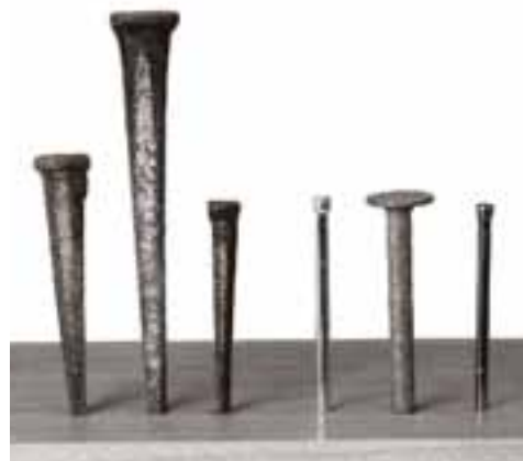
Cut nails (left) taper on two long edges and have rectangular cross-sections; wire nails (right) are straight and round.
