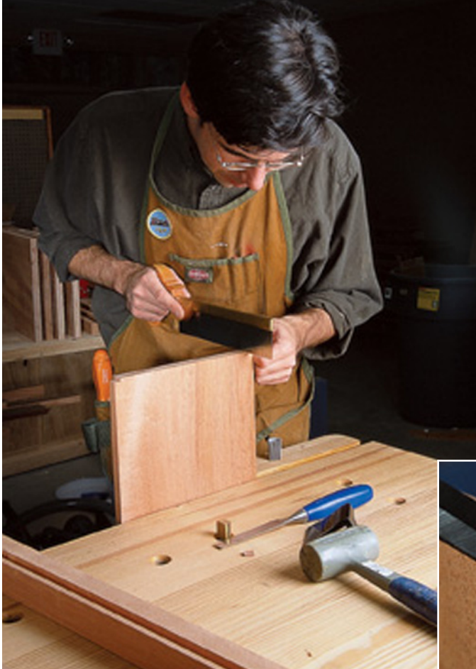
You'll need to notch the bottom of the side panel to fit in the leg groove. A backsaw makes quick work of this simple operation (above). Clean up the cut with a sharp chisel and you're ready to move on (right).
