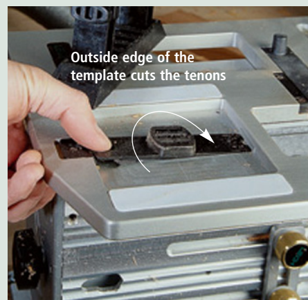
The templates snap in and out of place with fingertip pressure. Pick your tenon size and pop it in the jig.
