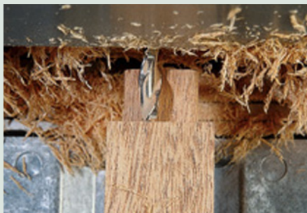
You can connect dust collection to the back of the jig, which I recommend. It doesn’t get all the chips, but it cuts down significantly on the mess.
