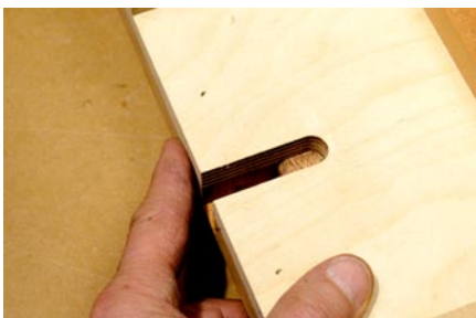
From below. The slot made in the jig is used to visually line up the jig with the router bit.
