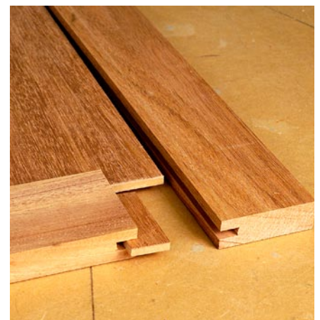
Tenon for the dust panel. A small piece of the plywood used for the dust panel is used as a loose tenon to hold the frame together.
