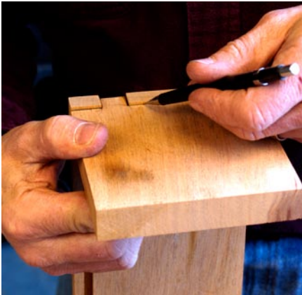
Getting the edge. To sand and pillow the proud fingers, first mark the limits of the pillowing with sharp pencil using the scrap drawer front
