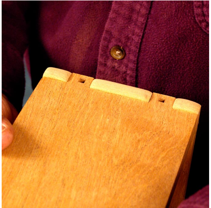
Results from careful work. After beveling, test the fit before assembling the finger joined drawer.
