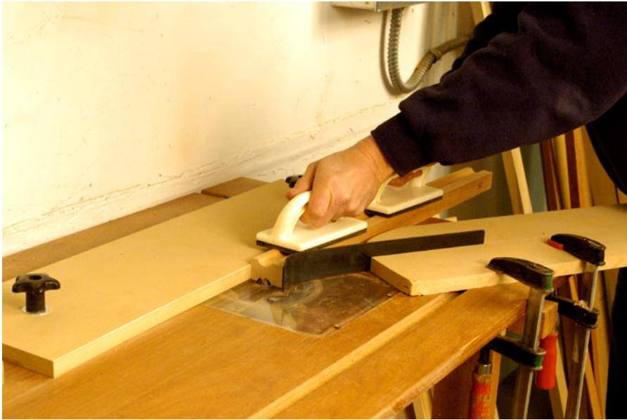
Fence matches handle. A curved piece of MDF is employed as a fence on the router table to guide the bowed handle over the core box bit, relieving the back of the pull.
