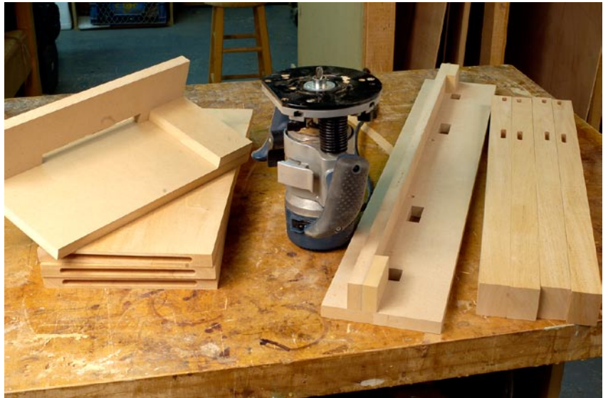
Templates for Tenons. MDF is used to make the templates for the loose tenons and splines. The router is fitted with a \frac{3}{4} " guide collar and a \frac{3}{8} "-diameter straight bit. Dry fit the template pieces before gluing to ensure that the collar will move easily in the opening.
