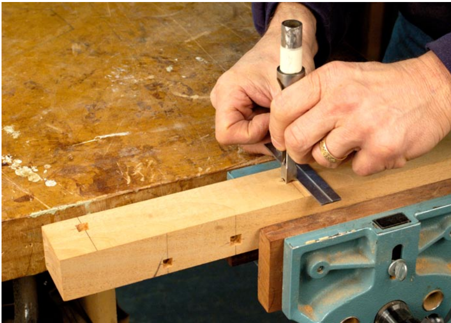
In position and in line. After locating the plug holes and drilling with an undersized brad point bit, a small square is used to position the hollow mortiser chisel. The points of the chisel will mark the spot.
