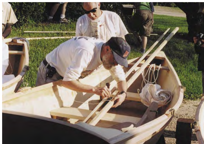
Merlin makes his boat ready for sail by attaching cord for lacing the sail to the mast. All the parts have come together for a boat, which now has oarlocks at two stations for rowing singly as well as with a passenger.
