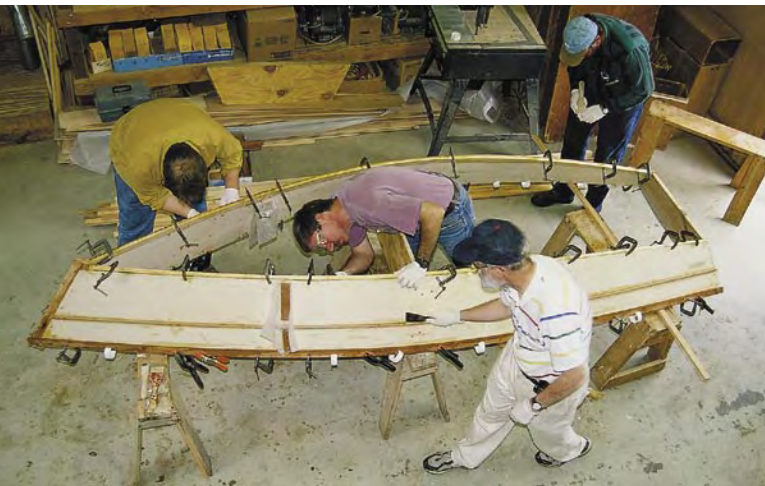
Single-unit design accomplishes the boat shape in one session. Less than three hours has elapsed since the epoxy was first spread. From left to right, Eisenlord, Hott, Merlin and Sarge clean the epoxy squeeze-out before it hardens. Note the use of 5-cent PVC clamps along with regular C-clamps.
