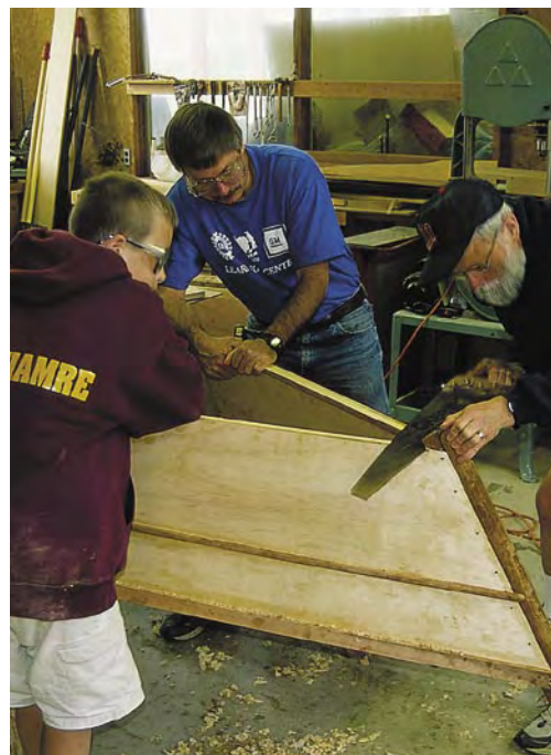
With the bottom ply cut to shape, and the chine logs planed flat, Lars and Hott hold the boat while Merlin trims the stem so that the bottom can go together.
