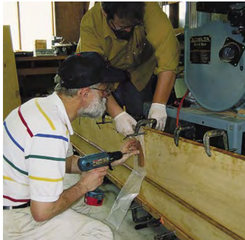
In a 12'-long boat, the plywood must be scarf jointed for length. The long beveled overlap joint uses scrap blocks on each side squeezed together with deck screws. Merlin (left) and Rick Eisenlord use waxed paper to prevent the blocks from being epoxied to the hull, as you see here.
