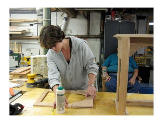
The four pieces that from the arch dial are glued. The half-lap joints provide a lot of gluing surface so no nails, biscuits, or screws are needed.
