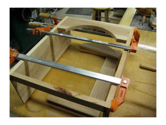
The tops of the clocks, the "hoods", are assembled and glued separately. They do not permanently attach to the waist - the appearance of a one piece clock is an illusion.
