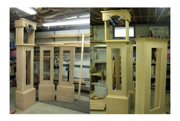
Here you can see clocks with the bases complete, cove molding attached, and one of the hoods sitting on top. At this point the clocks are really starting to take shape!
