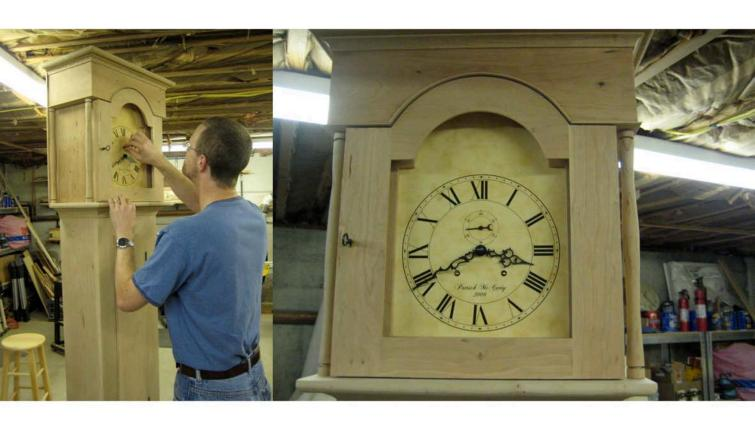
Final dry-fitting of my clock prior to the finish being applied. Keyhole grommets, though not called for in the plan, add a nice finish and help hold the paper face flat. The grommets were procured from a local clock shop. The grommets were a dollar, but the half-hour clock-movement lesson I got from the store owner was free!
