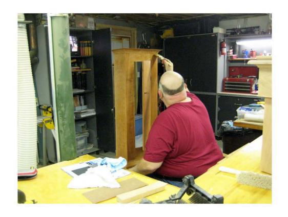
Clocks were finished in three steps. A sanding sealer helps to reduce the blotching inherent in Cherry.
