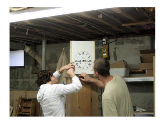
The movements were mounted to the seatboards and the clock faces were added, along with the hands. The faces are held fast by a dab of hot-metal glue in the corners, and keyhole grommets are tapped into the holes by a mallet.
