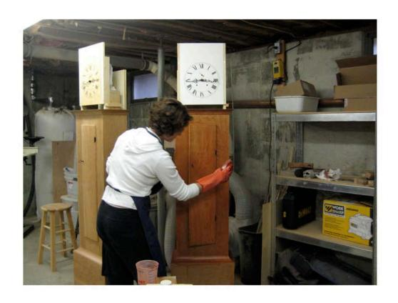
Erin applied an extra coat of the Danish Oil to her clock for a darker color. After the oil, the clocks received two coats of lacquer, sanded smooth after each coat with fine steel wool.
