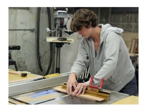
The arch frame is made with half-lap joints. Stock is removed using the table saw to nibble away stock one "kerf" at a time. This is a slow procedure but works well.
