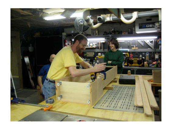
Like the waists, the bases were joined with biscuits and glue. Once the bases were dry, adjustable feet were attached and the bases were screwed to the waists.
