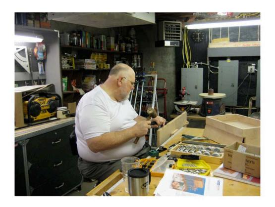
Here Tom is making final adjustments to one of the waist doors. Getting doors to fit properly with the hinges is deceptively difficult to do. In this case, a binding door was removed and the hinge mortises deepened.
