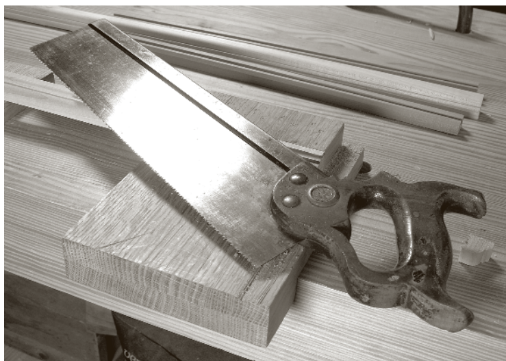
A classic vintage carcass saw from Wheeler, Madden & Clemson. This saw is 14" long and has 12 ppi. The carcass saw is used for almost all joinery cross-cuts when building furniture.
