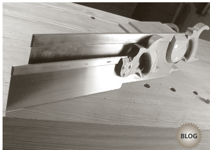
These two saws are so different in size that it's hard to believe that they both are called tenon saws. The big saw is a much older (and almost extinct) form.
