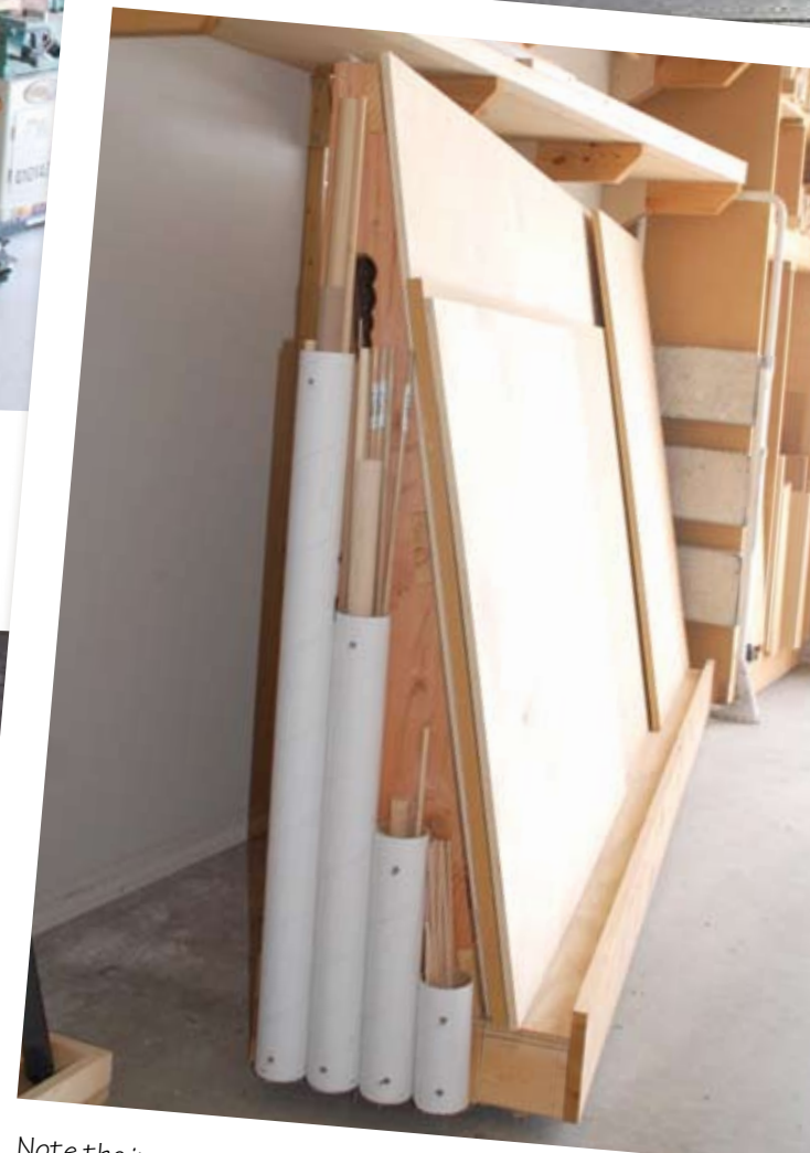
Note the ingenious (at least I thought it was at the time) use of mailing tubes for dowel rod storage.
