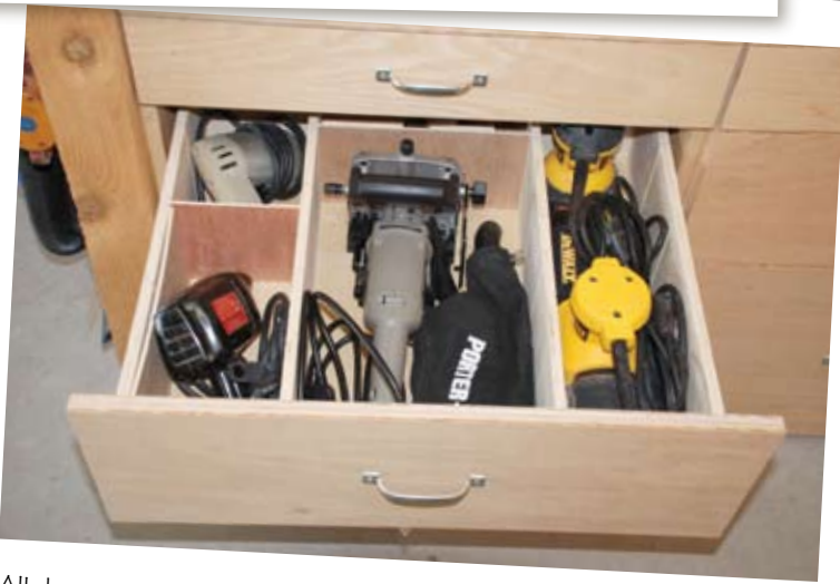
All drawers were designed and built utilizing removable dividers so they can be easily reconfigured as I add to my tool collection. Remember, every new project should require a new tool.
