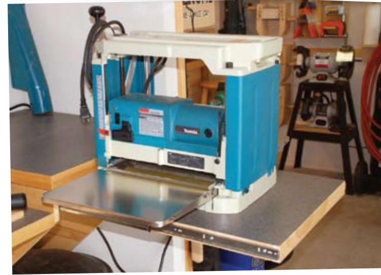
Smaller tools are stored within easy reach and set up as needed. I use a flat shelf which I pull out from under my miter-saw station to position the planer when needed. The shelf is on drawer slides.
