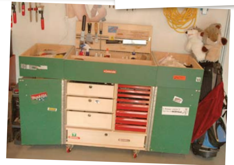
I built this rolling cart for the magazine and couldn't part with it. It stores the majority of the small supplies, sharpening, sanding and more. Tucked behind the left door is a benchtop drill press. Behind the right door (next to the clubs) is a small combination belt/disc sander.
