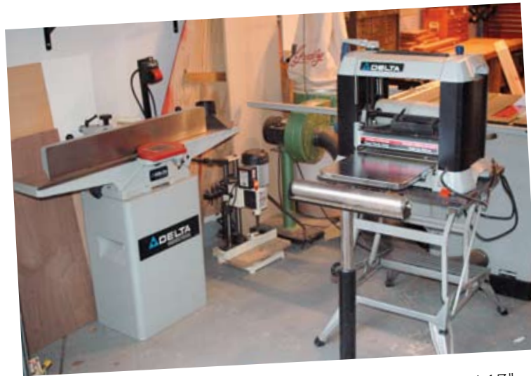
While not the size equipment I'd love to have, a 6" jointer and 13" portable planer (with roller stand, very important for a one-person shop) can handle the great majority of woodworking tasks. A Grizzly dust collector hooks to the tool in use at the time. Conveniently, the small shop space makes it only necessary to shift the hose. And yes, there's a mortiser tucked away in the corner.
