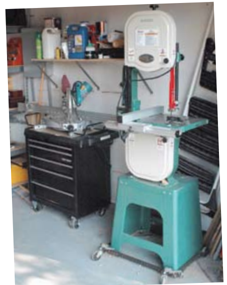
A 14" bandsaw (on wheels) and a 10" sliding compound miter saw with fence extensions (on a great rolling storage cart) share space with the "garage" storage shelf above.
