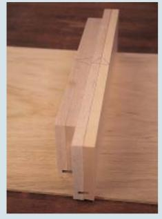
**Step 1** Lay out all the drawer parts in order, and label using an orienting triangle. Remember that the drawer sides will capture the front and back when the drawer is assembled.
