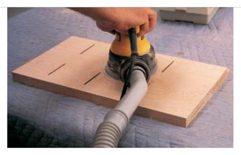
After the slots have been cut and you've determined that the parts fit together properly, finish sand all the parts. Cover the slots with masking tape, and finish the parts.
