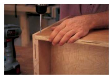
The back is screwed to the base. Note that the screw is inserted at a slight angle so it won't cause a bulge on the inside of the project.
