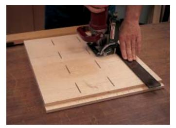
Lay the two side panels side by side and cut all the biscuit slots at the same time. This will ensure that the shelves will be level and the project will be square when assembled.
