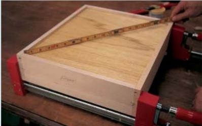
**Step 4** Assemble the drawer. You can either use a captured bottom (as shown here) or cut the bottom of the back part off. The bottom can then be slid into the assembled drawer after the drawer and bottom have been finished.
