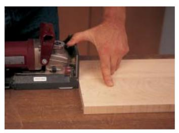
2 | Lay the shelves faceup on a flat surface when cutting the slots.
