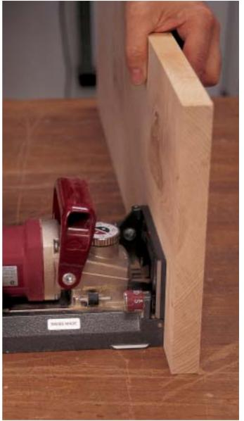
Stand the top on its back edge and cut the slots that line up with the back panel. Next, cut the slots in the top where the sides will attach to the top, using the layout square. To locate the slots, dry assemble the base of the project and measure the distance between the slots in the tops of the sides. Transfer this measurement to the top panel, making sure the top will be centered on the base.
