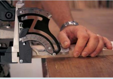
**Step 2** Mark the location of the biscuits and cut the slots in the front and back parts. When making drawers, use the largest biscuits you can.
